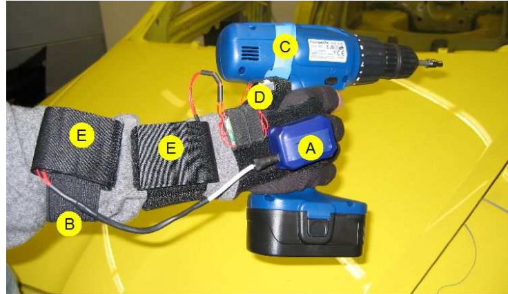
Fig. 2. Wearable sensors attached to the dominant hand of the worker
