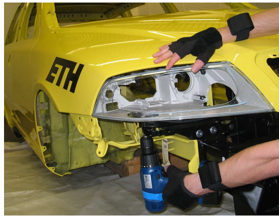
Fig. 1. Front part of the car body where the lamp is assembled
